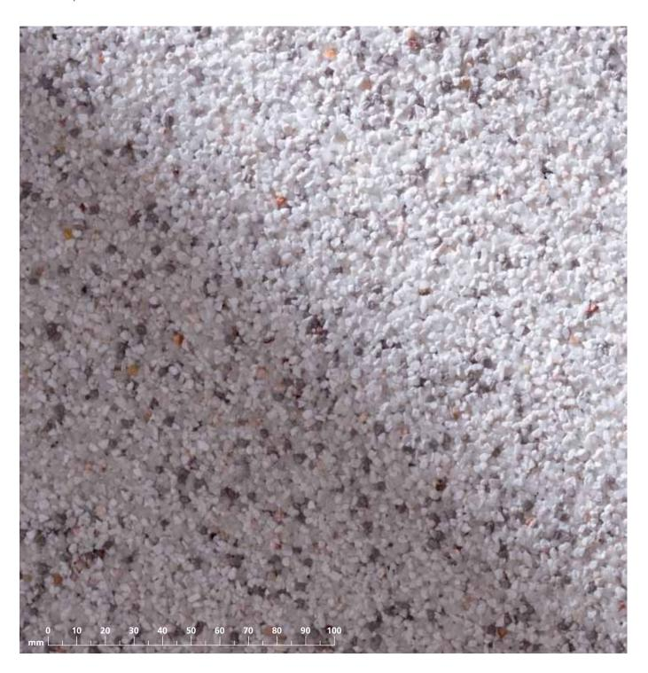
An attractive, multicoloured finish with a heavy texture and natural stone aggregate, ideal for high impact areas and splash zones below the damp-proof course. Available in 13 aggregate colour combinations, the finish can be used for selected areas or over the entire elevation.
