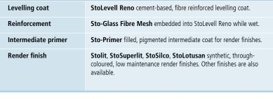
StoRend Fibre Plus is a high quality render system from Sto using a fibre reinforced levelling coat combined with a tough, flexible reinforcing mesh to yield exceptional levels of crack resistance.
