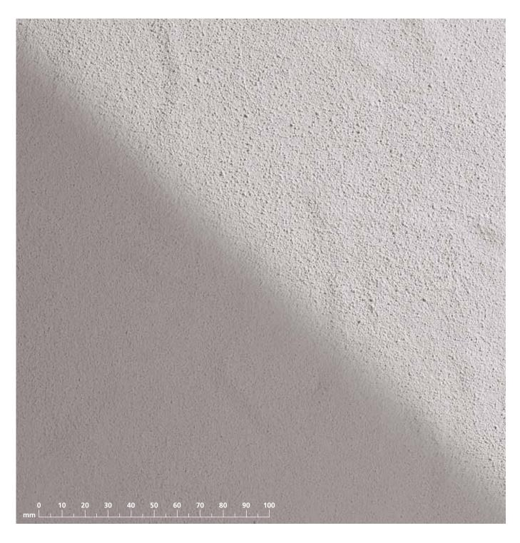
If a unique, bespoke facade finish is required, MP renders are the ideal solution. The material can be rubbed up to give a near smooth texture or provide a variety of textures for the facade.
